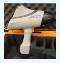
Handheld X-ray Fluorescence (XRF) Spectrometer for analysis of elements in metal alloys.
