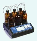
**Respirometer** for measurement of biological oxygen demand in water.
