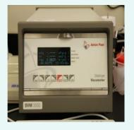
Stabinger Viscometer for kinematic viscosity of transparent and opaque liquids.
